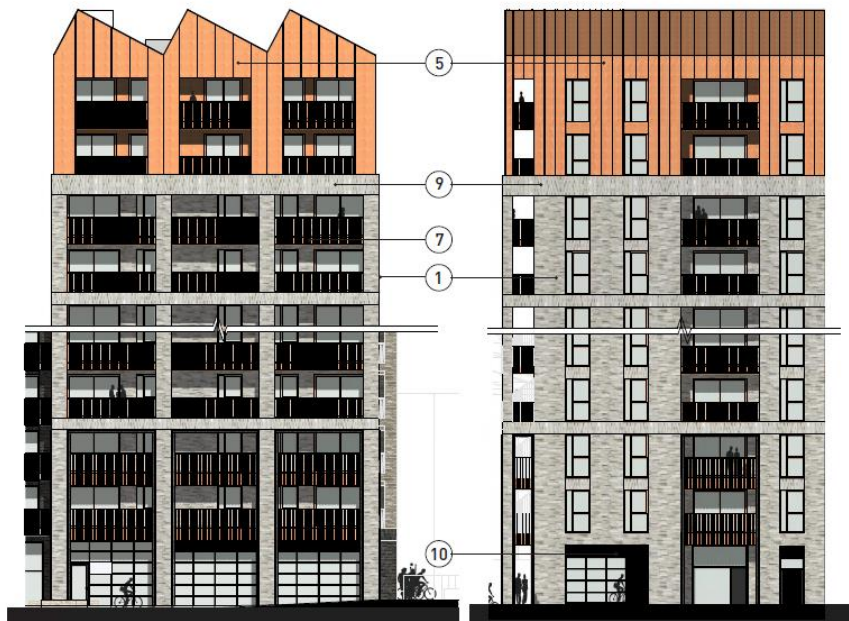
Figure 10: Tower A1 (Part south and east elevations)
